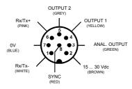
NOTE: the wire colours refer to the cables manufactured according to the European standard
