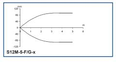
The operating distances indicate the detection distance with excess gain 2.
