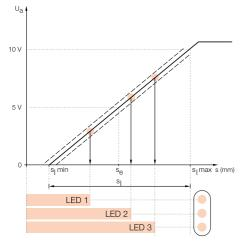
With sensors having the teach-in function the switching distance can be freely programmed within the working range. This can be done either using the BES 516-4 programmer (starting page **6.2** ...) or directly on the control line of the sensor.
