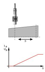
Detecting larger travel by sensing an inclined surface.
