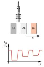
With the distance constant, the output signal will change only of the object material changes.
